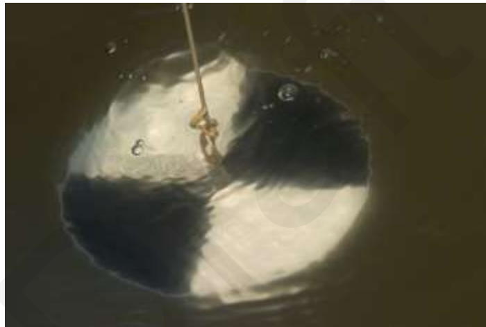
Figure 11 – Black and white Secchi disk for measuring water clarity
